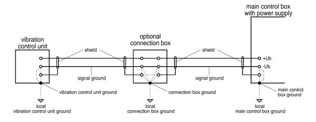
If an isolated installation is not specially requested, usually through the attachment with screws each case is connected to the local machine ground.
