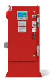
**Description** – Firetrol\* FTA1000 Full Voltage Fire Pump Controllers are intended for use with electric motor driven fire pumps where the capacity of the power source permits full voltage starting. Full voltage is applied to the motor as soon as the controller is actuated. The controller monitors, displays and records fire pump system information.
