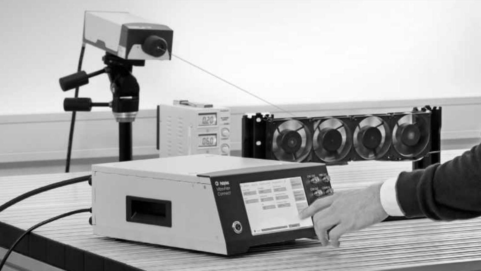
Core of VibroFlex as flexible laser vibrometer solution is the front-end Connect. Its latest generation FPGA-based signal processing takes care of decoding raw measurement data in displacement, velocity and acceleration, signal conditioning and data interfacing (analog and digital). The front-end Connect enables custom setups and makes sure to have the application-specific settings
