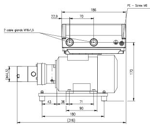
recommended installation position: drive shaft horizontal
