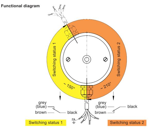
Switching occurs by rotation to the right, clockwisely, when looking at the front-side (cover with screws).
