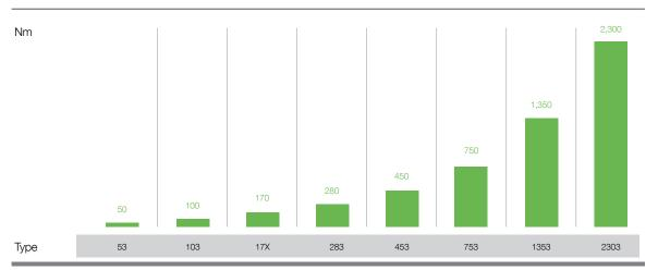
Output Torque of Parallel Shaft Gearboxes
