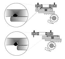
The **Soft Seat Valve Seal** is available for all DBB Orifice Fitting models. Effective in all scenarios, this unique design enables a bubble-tight seal between the three chambers without the need for frequent valve lubrication. The specially machined seal channel helps prevent O-ring dislocation, and the O-ring seals incorporated are available in a wide variety of compositions. The DBB Orifice Fitting is also effective with standard grease seals.
