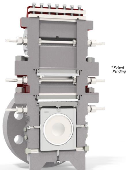
Designed after HSE HSG 253 Cat 2 Isolation, and built to meet or exceed ASME and ANSI specifications, as well as to comply with the latest editions of AGA-3 / API 14.3 or ISO 5167, the Canalta DBB Orifice Fitting provides accurate flow metering over a long service life and superior protection from high pressures and toxic flow media. Available as fitting only, retrofit or complete AGA-3 or ISO 5167 compliant meter run.
