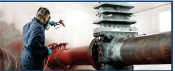
Each Canalta Single Chamber Orifice Fitting receives a standard coating that includes a non-lift oxide primer and fast-drying enamel finish in Canalta Grey. Custom coatings for special environments - maritime, humid, high temperature and others - custom colours and primer only applications are also available.
