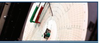
Our comprehensive *Quality Management System* includes full function, hydrostatic and pneumatic pressure testing to prevent defective orifice fittings from reaching service. Standard testing comes at no extra charge and includes verifiable pressurization to 150% of working pressure. Additional inspections, such as radiography, ultra sonic and liquid dye penetration, are also available.
