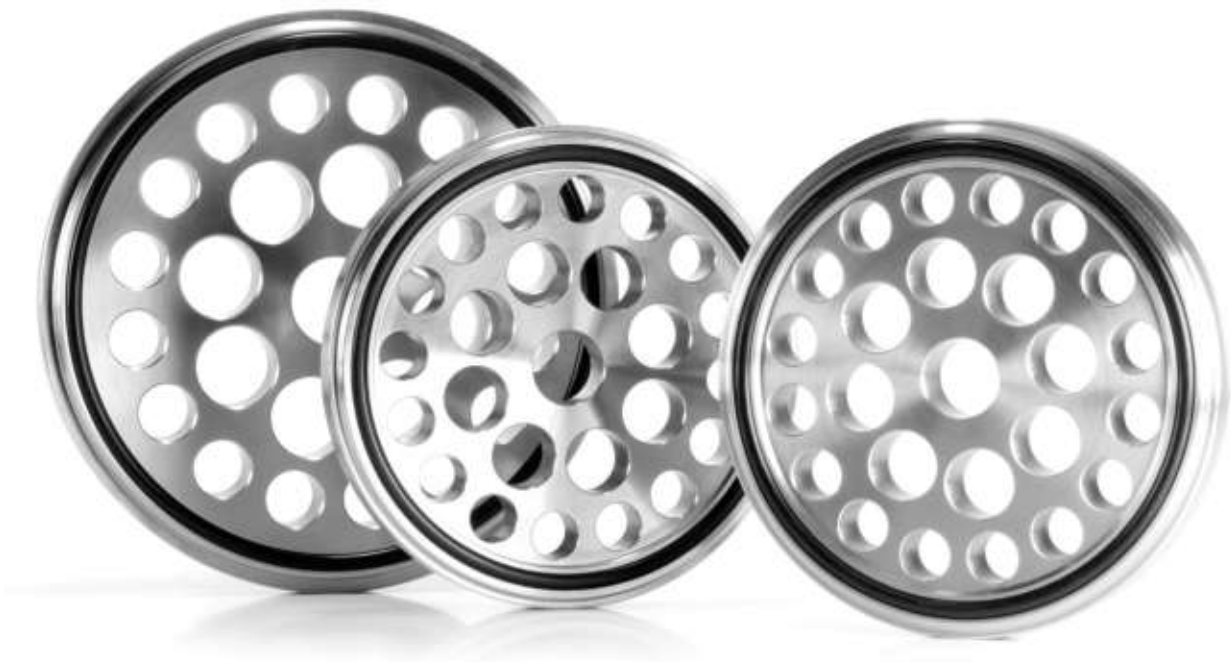
Canalta's Contour™ FCH Flow Conditioner Housing lineup utilizes a newly designed flow conditioning plate. These isolating flow conditioners incorporate a non-protruding HNBR seal around the downstream face to prevent bypass leakage and protect the integrity of the flow profile. Available in a variety of plate geometries, including Contour™ K5, Zanker, Spearman and others.
