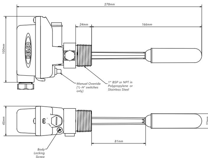
The switch requires a minimum of 25mm of clearance above and below its centre line axis to facilitate the free movement of its float.
