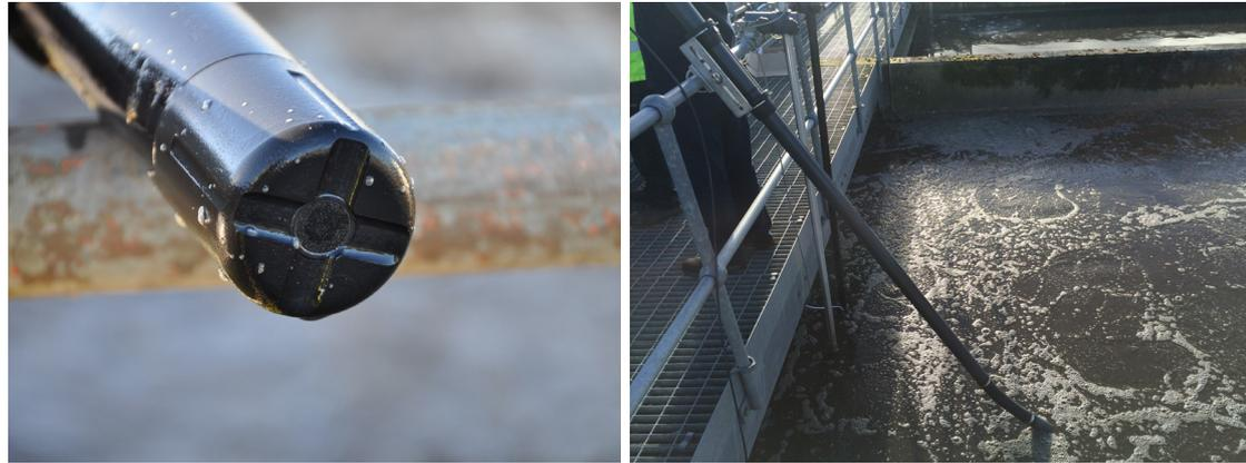
The OxyTechw<sup>2</sup> RDO Pro-X Sensor uses the latest optical technology for measuring dissolved oxygen (DO) in demanding wastewater, drinking water, industrial effluent and surface water environments.
