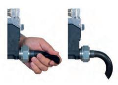
The engine wall screw fitting with its flexible intake funnel is mounted from the outside. Its form prevents splash oil from being drawn in and a false alarm being triggered. We can offer you a suitable engine wall screw fitting to match the engine wall thickness.
