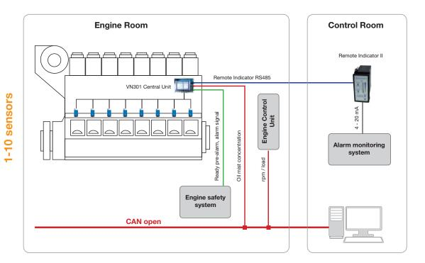
sensors ensure that the crankcase is monitored.
